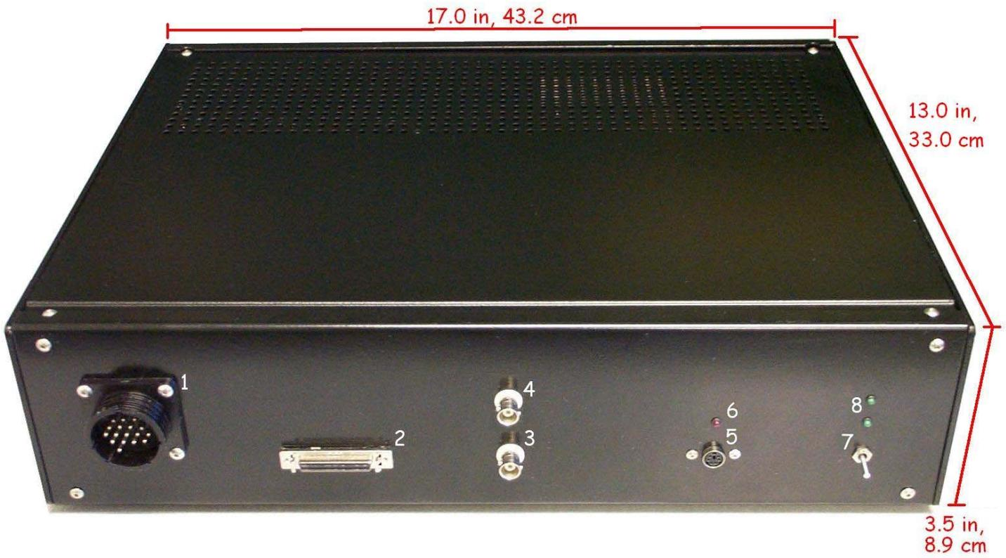
Figure 1: Thermal Transient Anemometer
